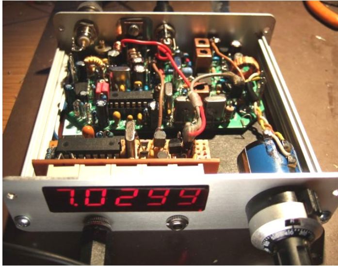
Miss Mosquita A 40 meter CW Transceiver So small – so spicy – it must be a Lady
